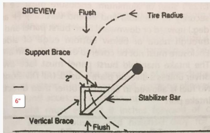
10. Mini Rod tractors must meet general tractor shielding, safety criteria and driveline shielding, with the following addition for vehicles with 8-71 or larger supercharger and/or planetary rear end.
